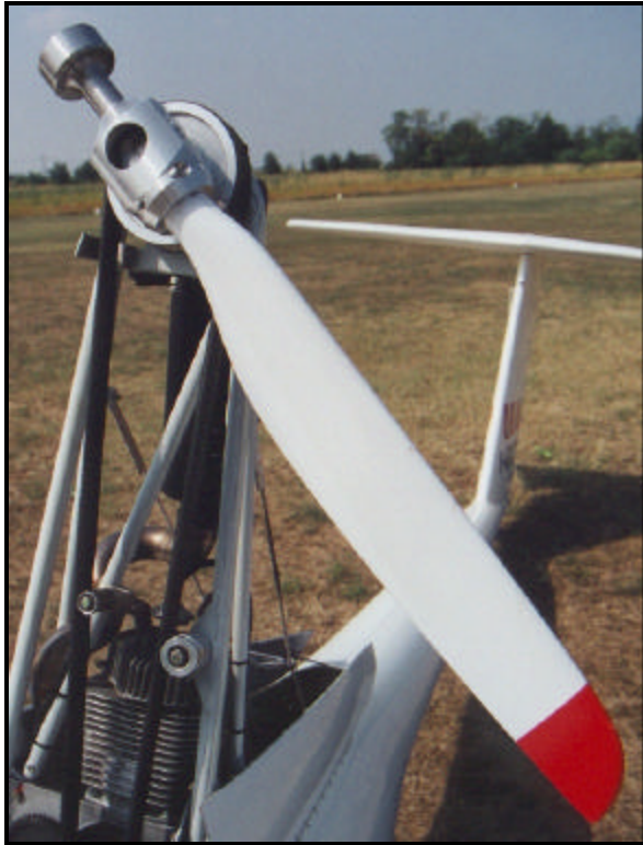
Patented single-blade teetering propeller.
