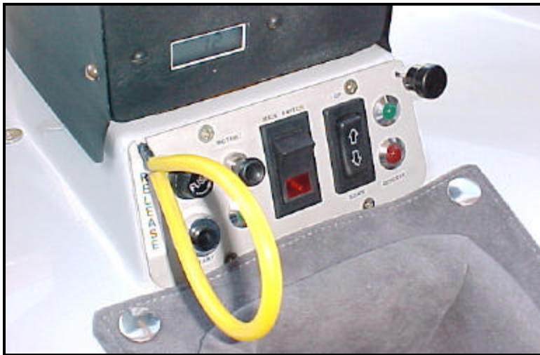
Silent-IN panel – indicator lights, pylon up/dn, master, ignition, & start.
