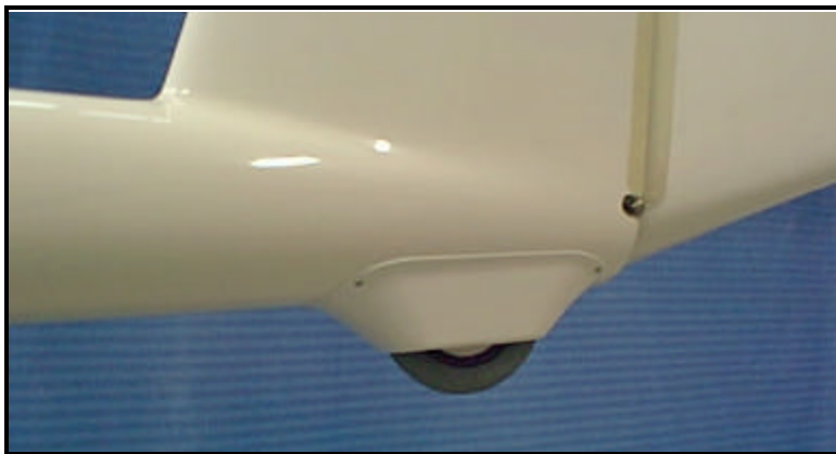
New version of the steerable tailwheel.
