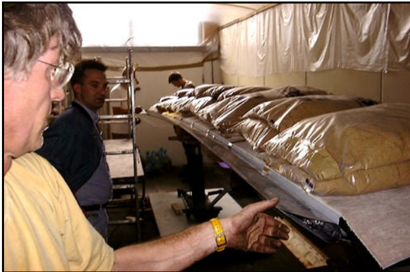
Wing load test with free movement of flaperon – booth heated to 54°C.
