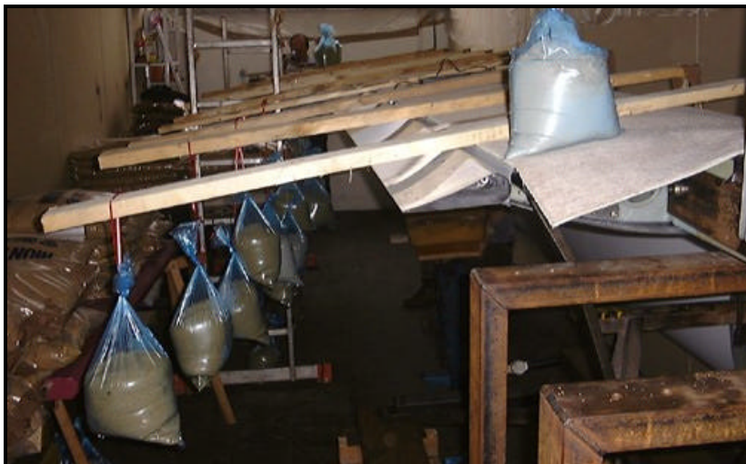
Wing torsional bending test.
