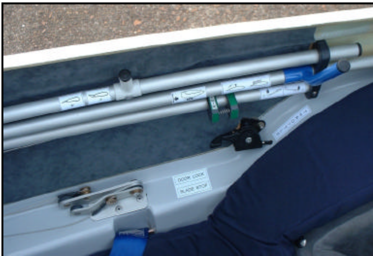
Cockpit side controls – door lock and blade stop next to seat harness.
