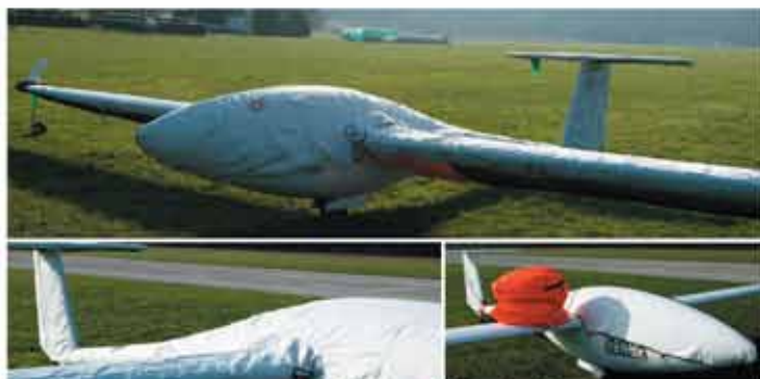
Protective covers Wing and fuselage protective covers protect all exposed surfaces from inclement weather, UV
