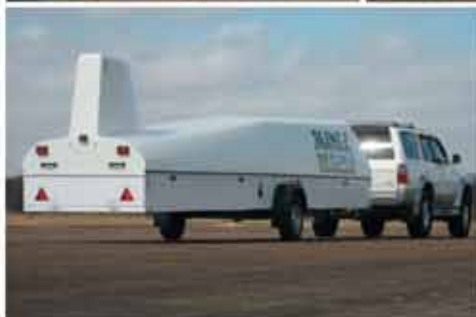
Protective covers Wing and fuselage protective covers protect all exposed surfaces from inclement weather, UV
