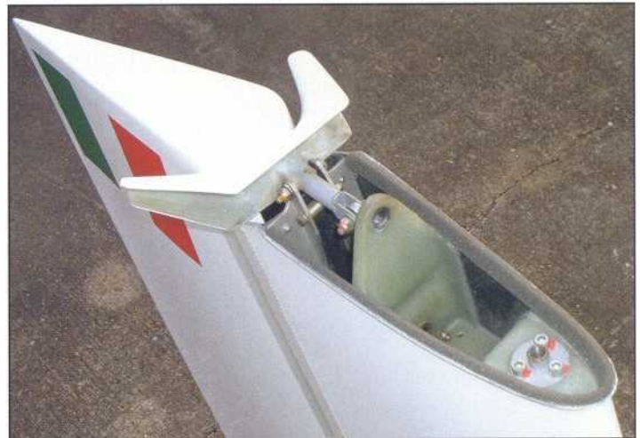
Elevator automatic control connection.
