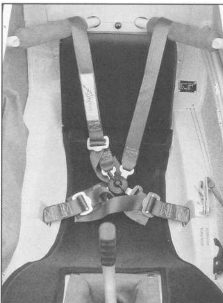
Quick release harness: one piece shoulder strap loops under the wing brace tubes.
