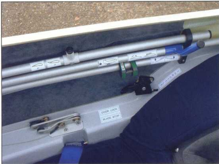
Controls (top to bottom): flap, airbrake, trim, throttle, blade stop, and door lock.
