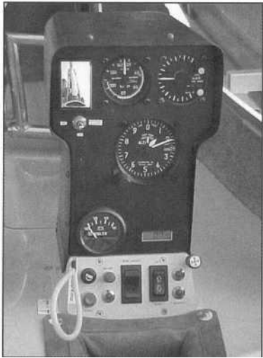
The pylon/engine control switch panel is located at the base of instrument pod.
